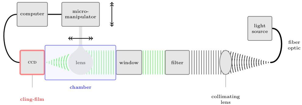
Figure 1: An illustration of the optical setup used to measure the point spread function (PSF) of marine animal lenses. While the cling-film protected CCD registers focused images of the point source, the computer controls the axial distance of the biological lens submerged in the chamber. By scanning the focal point the optimal focal distance was estimated. All the dimensions of this setup are mentioned in the text.
